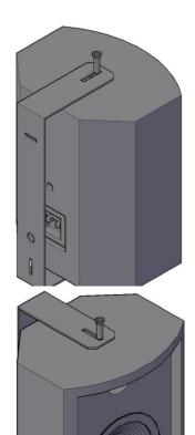
ARC115 speaker can be mounted on the wall or roof using its own bracket.
