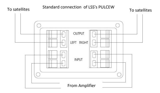
Usually PULCEW works well with PULCE speaker, an example of recommended configuration using multiple with PULCEW in STEREO Mode speakers is represented below:
