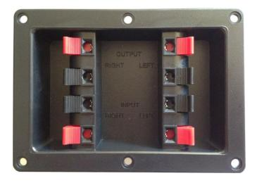
Considering only two couples of Black and Red clamps (right or left), the bottom couple is the input, the upper couple is the output.
